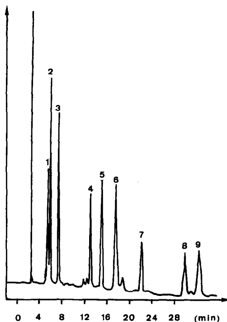
Fig. 6. Separation of a standard mixture of nine carotenoids by NARP-LC. Column, Zorbax ODS (250 × 4.6 mm I.D.); mobile phase, acetonitrile–methylene chloride–methanol (70:20:10, v/v/v); flow-rate, 1 ml min -1 ; detection, 450 nm. 1 = Lutein; 2 = zeaxanthin; 3 = canthaxanthin; 4 = \beta -cryptoxanthin; 5 = echinenone; 6 = lycopene; 7 = torulene; 8 = \alpha -carotene; 9 = \beta -carotene. From ref. 71.
